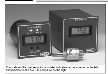
The Vacuum Research pressure gauges are compact pressure measurement and control instruments that offer the precision and high resolution of digital electronics at the same price as analog instruments. These instruments use a rugged and stable silicon diaphragm type transducer with an 1/8 inch NPT connection in a stainless steel housing.
