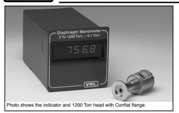
The Vacuum Research Diaphragm Manometers are compact vacuum measurement and control instruments that are unaffected by gas composition. The sensors have 316 L stainless steel diaphragms and any sensor can measure liquid or gas pressure as well as vacuum.
